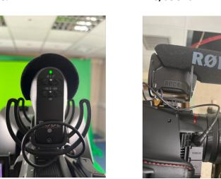
5. You can use the camera's own built-in microphone or the microphone on top of the camera. If you use the second one, please make sure that the cable is connected to the camera and switched on. You will need to adjust it according to the tone of voice of the person being recorded.
