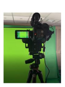
4. Adjust the camera position and distance, depending on the height of the person you are recording, by moving the tripod and camera.
