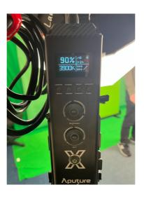
2. The lights should come on automatically and they have a set setting. 90% and 3900K. If not, adjust the lights using the controls.
