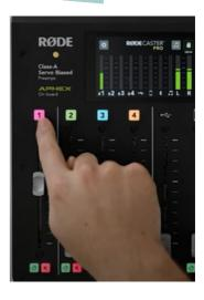
3. Press the channel button to go into the settings for this channel
