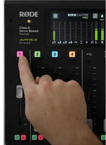
3. Press the channel button to go into the settings for this channel
