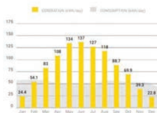
Figure 28: Aras Spraoí (Scenario 2) PV Array Installation & System Performance, Open Solar
