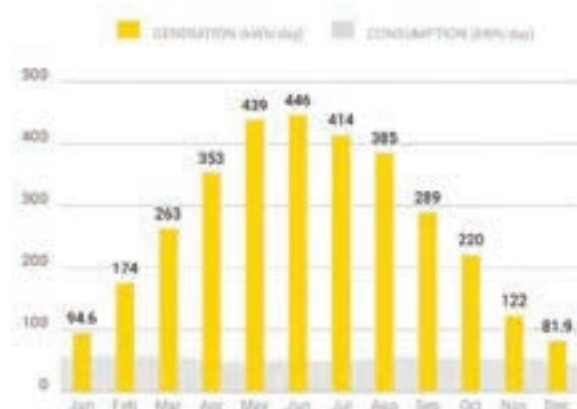
Figure 27: Aras Spraoí (Scenario 1) PV Array Installation &amp; System Performance, Open Solar
