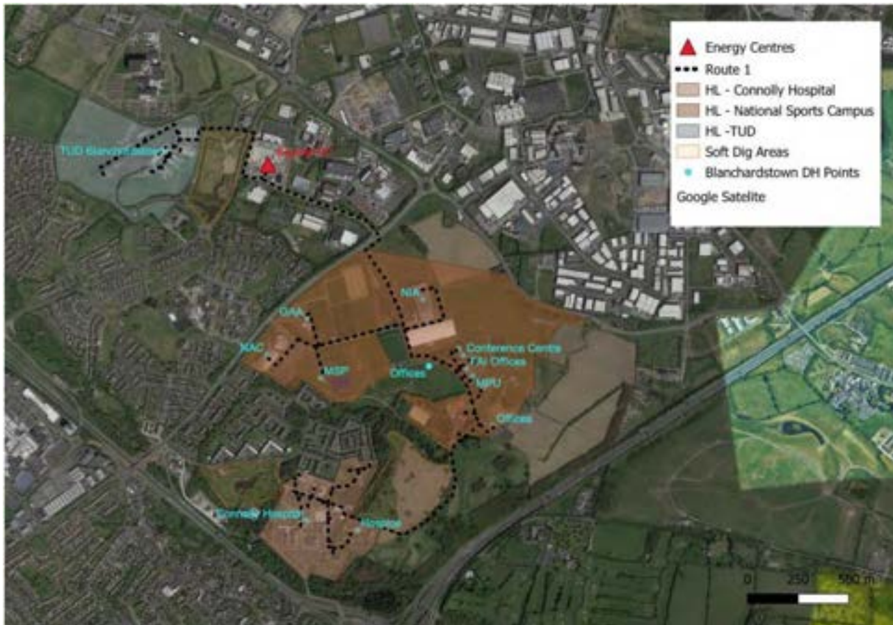
Figure 25: One of the three potential routes considered in the Outline Business Case of the Blanchardstown district heating system showing the pipe network between the data centre and the TU Dublin Blanchardstown Campus.
