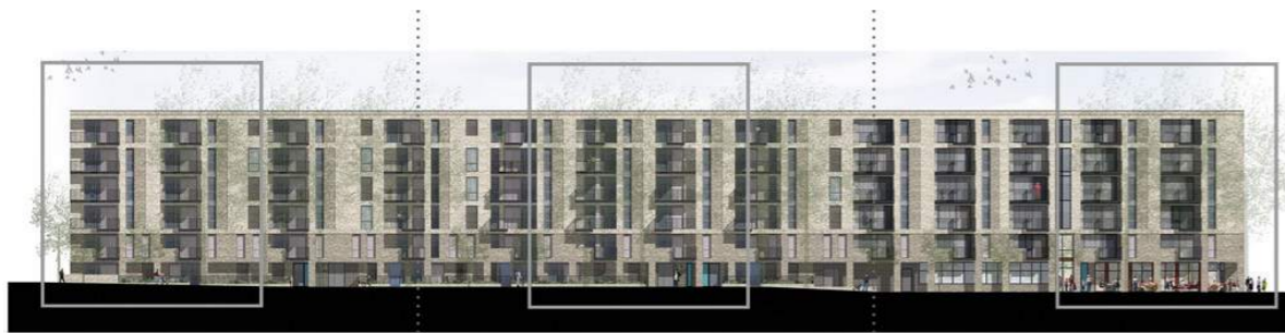
The three different cores for the three different tenure types at Lime Tree Court and how it is reflected in the facade
