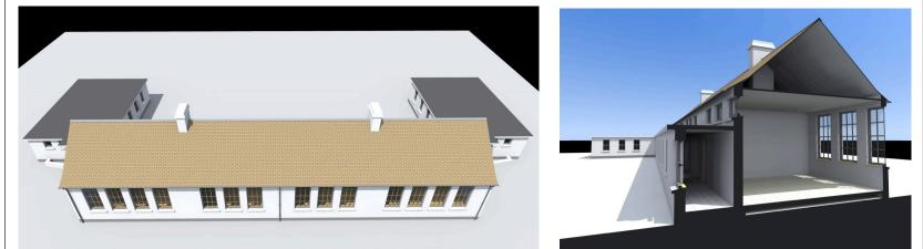
The energy performance of the existing school building was examined and calculated using the PHPP spreadsheet software as well as a range of other analysis tools and methodologies such as Design Builder (Dynamic Simulation Software), U-Value calculation software (Build Desk-U), Linear Thermal Bridge Modelling (Therm), and Hygrothermal Moisture Assessments for Surface and Interstitial Condensation.
