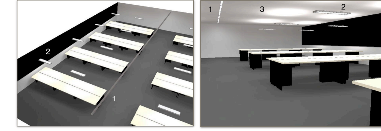
Daylighting Strategy: (1) Glare zone (desk work areas set-back from perimeter), (2) Office working areas with good daylight distribution (200-300 lux), (3) Circulation and ancillary spaces to central zones with lower daylight levels (<200 lux).
