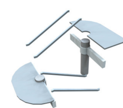
Metal supports for stairs placed on the cast in-situ concrete floor supported by structural frame
