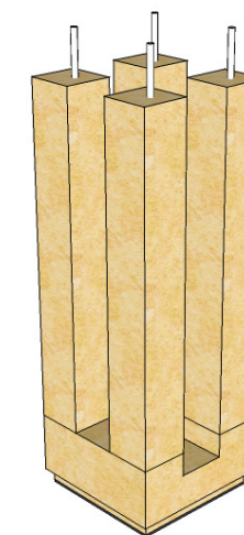
Step two is when the four supports are connecting to the base stone by the steel pins and epoxy resin.
