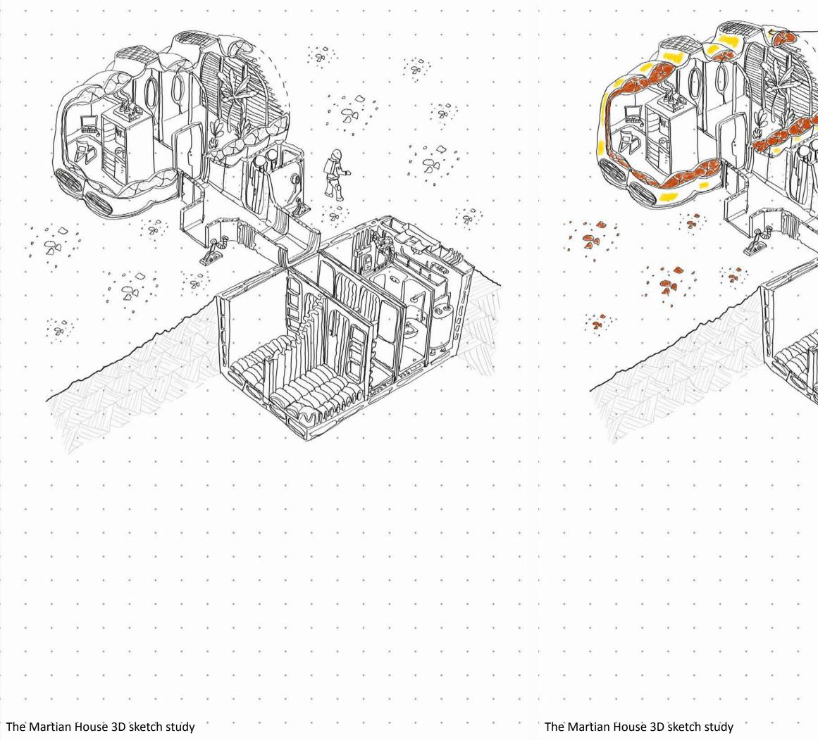
GOLD RIPSTOP NYLON FABRIC LIGHTWEIGHTINFLATABLE ROAMWORK MARTIAN REGOLITH BONDED WITH BACTERIA INFILL 43
