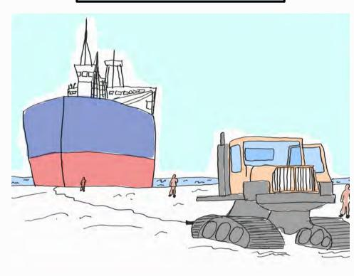
The components of construction were delivered to Antarctica in a giant ice-strengthened Russian cargo vessel - the Anderma. Bow and stern lines were moored in the sea ice. Mooring points had to be prepared in advance of the ship's arrival. These entailed excavating 2 m deep holes into the ice and setting timbers into the excavation with anchor ropes extending to the surface. The holes were refilled with compacted snow which then refroze, providing secure mooring points.
