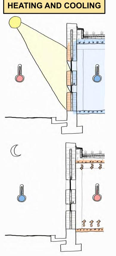
In-slab radiant cooling and heating in both ceiling and floor slabs create an even, comfortable environment that avoids blasts of air, noise and dust. Coupled with 100% outdoor air displacement ventilation, the system will result in savings of 30 to 50% over a forced-air system.
