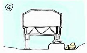
A hydraulic leg is lifted on one side of the module.
