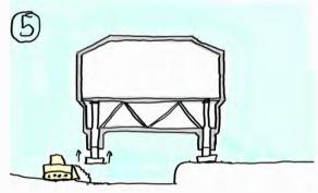
The hydraulic leg is lifted on other side of the module.
