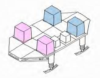
Stage 5: Prefabricated pods are installed onto the floors of the module. The pods installed include fuel tanks, generators, bedrooms. bathrooms, etc.
