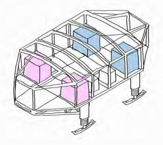
**Stage 6:** Steel superstructure is fitted over the pods, ready to receive the cladding.
