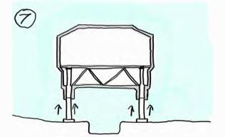
Once each leg is under a pile of snow, the module is raised by the hydraulic legs.
