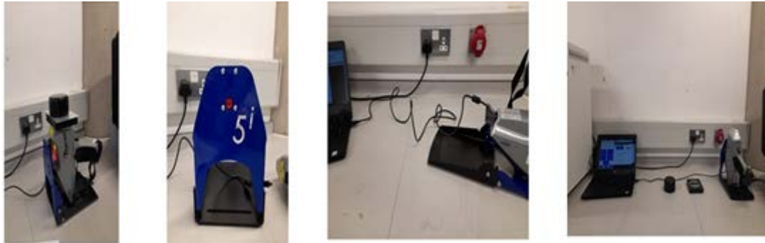
XRF orientation Release button XRF connected to Laptop XRF > 1m from laptop
