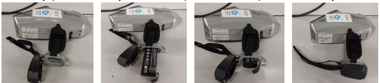
Figure 1. Insertion of battery in TRACER 5i XRF.
