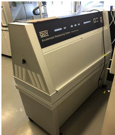
Figure: QUV Accelerated Weathering tester
