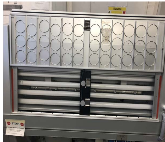
Figure: QUV Accelerated Weathering tester
