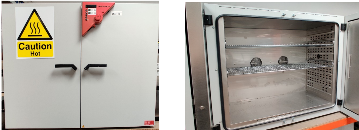
Figure 2: Large programmable composite oven with access port to maintain vacuum during cure.
