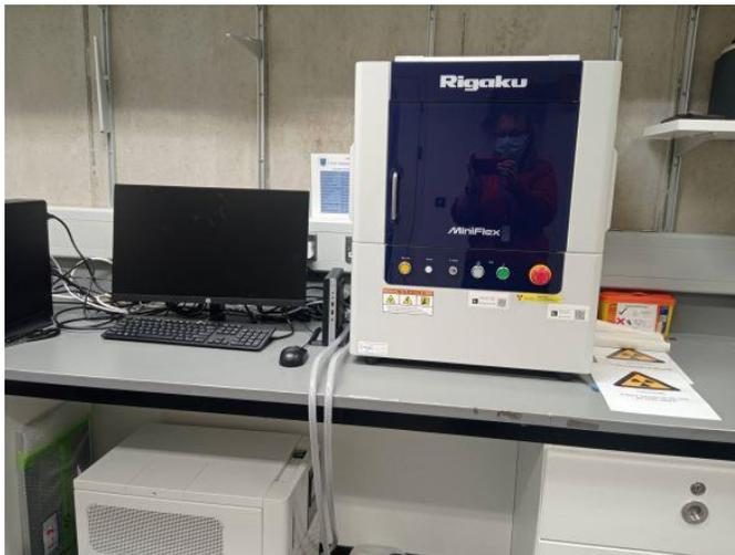
Figure: Rigaku Miniflex 600 Benchtop XRD
